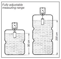
between 90 and 200 cm. All measuring ranges provide a full scale reading of 270°. Indication in percentage (height). A litre scale may be retroUnimes is the only mechanical contents gauge with litre scale facility.
